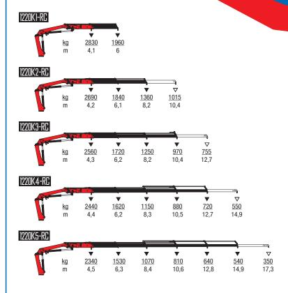
▼ Lifting capacity without manual extensions∇ Lifting capacity with manual extensions
