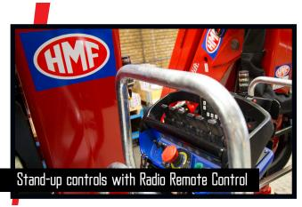
With stand-up controls and radio remote controls the crane operator has an increased overview of the crane movements. The remote control is placed in a bracket on the stand-up platform where it is fixed whilst operating the crane. The crane operator is protected by the HSL or HSL-E safety system which prevents the crane from hitting the operator on the stand-up platform.
